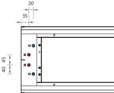
cooling and heating: 4 x Ø 12 mm
