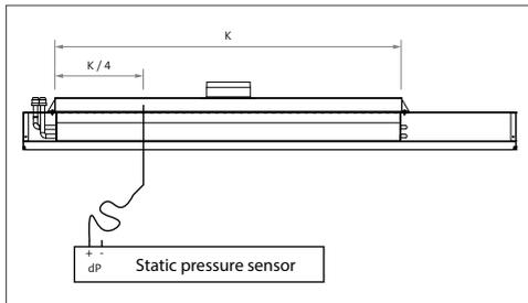
This requires a thin tube that is inserted through the nozzle into the plenum. Remember that for extravent units you use an open nozzle to carry out the measurement. Inserting the measuring tube in a closed vent could damage the seal of the extravent strip and produce noise problems.
